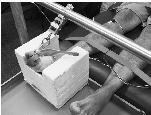
FIGURE 1—Great toe harness and strain gauge attachment.
